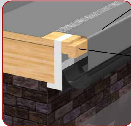
**A170/A200/A250 - Drip edge trims** Drip edge trims are fitted to the lowest edge of the roof where the rainwater flows into the gutter. To ensure the vertical leg of the trim sits into the centre of the gutter, the trim needs to be packed out by using two support battens, the first fixed just below the level of the deck and the second 10mm below the first, to allow the trim to sit flush with the roof.
