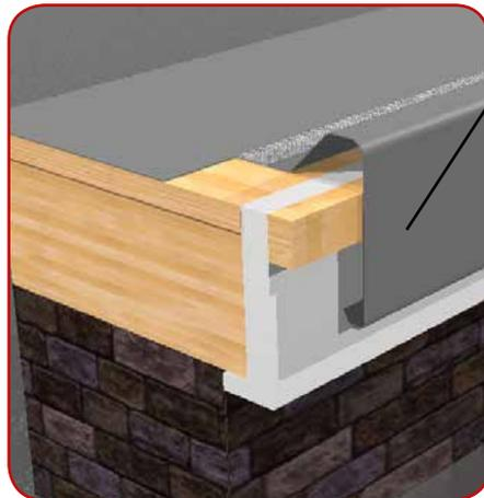
**B230/B260/B300 - Upstand (raised edge) trims** Upstand trims are placed on the non-draining open edges of a roof, overlapping onto the fascia boards. A single batten should be fixed on the outside of the fascia board level with the top edge of the deck. Cromar PU trim adhesive should be applied to the battens in 30mm beads at 300mm centres before bedding the trim.
